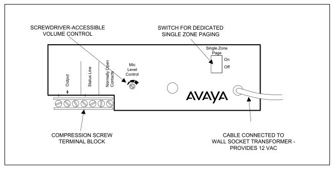
Figure 2. Back Panel Controls and Connectors
